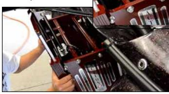
NOTE: It may be necessary to install the wiring harness before bolting the motor to the jack plate. Move the jack plate up for clearance to install the motor to the jack plate.
